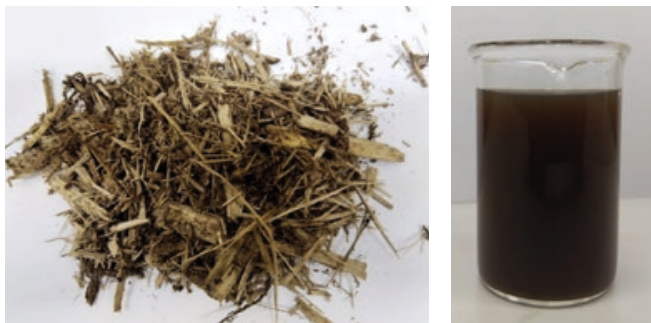
Figure 3. Spruce bark (left) and tannin extract (right) developed by University of Oulu for use as biocoagulants.
